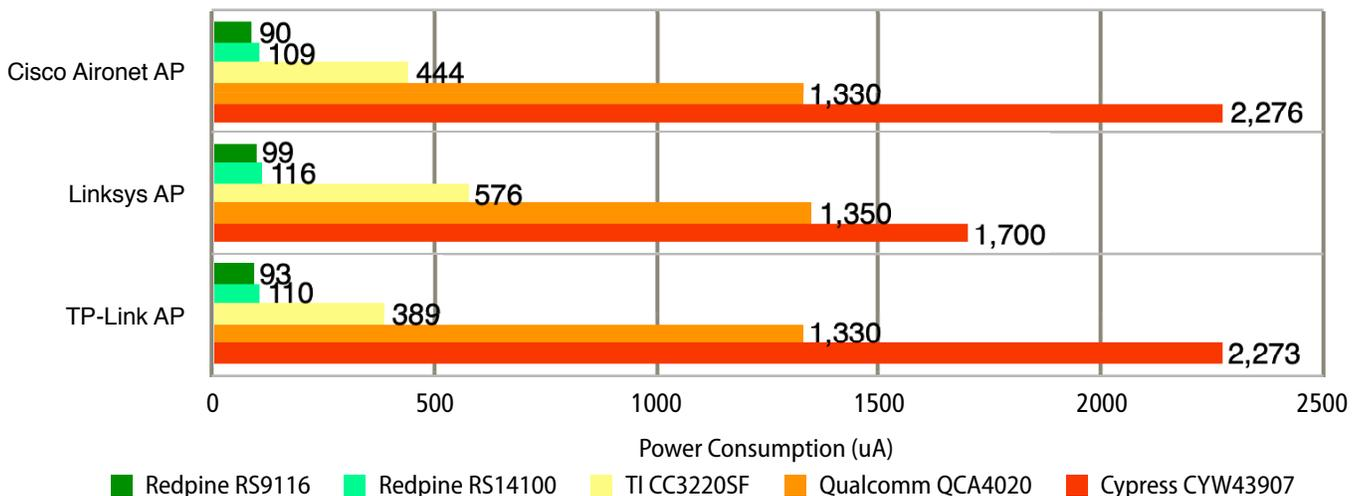
Notes: Tests conducted using vendor evaluation kits. AP DTIM set to 3. All testing using 2.4GHz band. See Table 2 for AP details.
